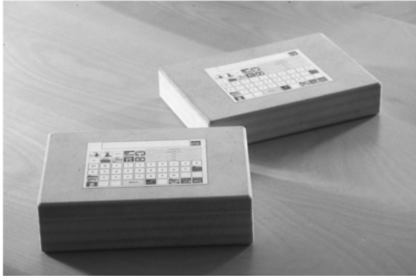
Figure 5.4. Block-level prototypes that are precursors to the DynaVox System's DynaMyte Augmentative Communications Device designed by Daedalus Excel Product Development. (Reprinted with permission of Daedalus Excel.)
